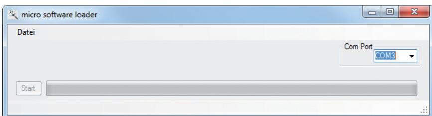
If you are not sure which port to use, check the COM port in the "Select Port" window in the "Menu" of the "Firmware\_Up-grade\_grStudio" and note down the COM port number for the "Silicon Labs CP210x USB to UART Bridge" entry – in this case "COM03". (If you select the wrong port, you will be alerted to this when you read out the receiver data). Click on "File" to load the corresponding firmware file named e.g. "GR12\_33577\_V\_XX.bin" from the hard disc ("XX" stands for the version number).
