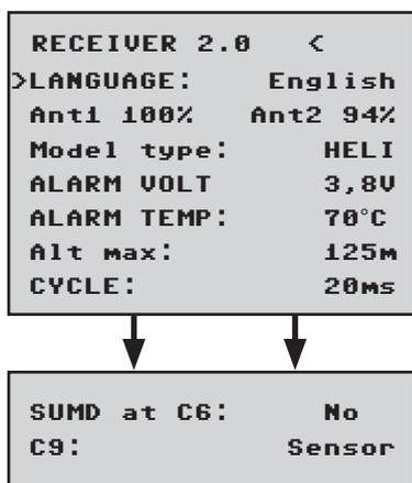
The receiver setup menu appears in the "Telemetry" menu under SETTINGS / DISPLAYS or if you are using a SMART-BOX under SETTING & DATAVIEW. How to access this menu is described in the operating instructions supplied with your transmitter or Smart-Box.
